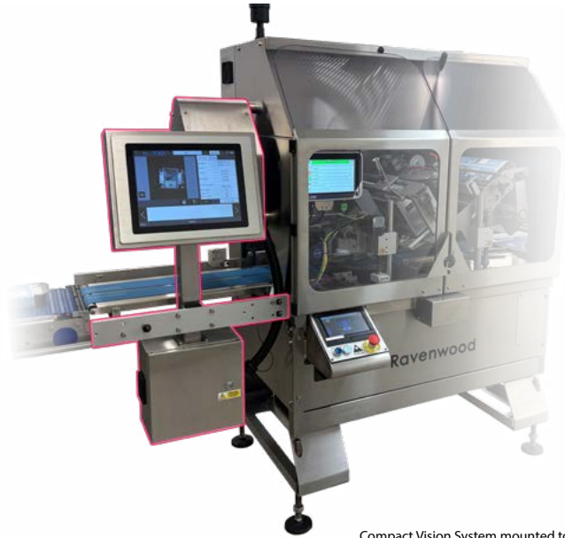
Compact Vision System mounted to a Nobac 5000 outfeed belt
